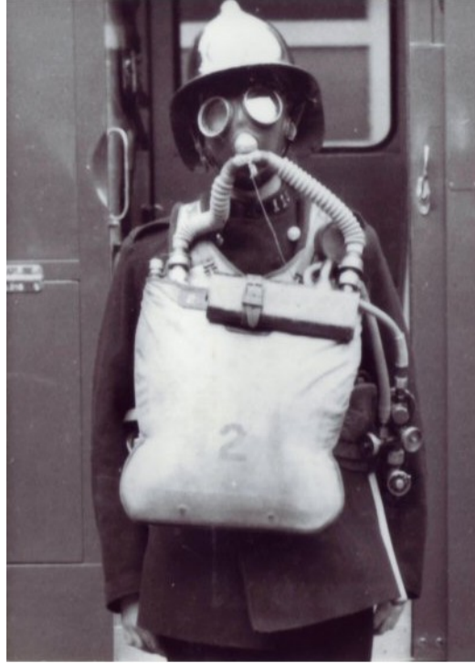
Fig. 6 Proto BA worn correctly SFB Photograph courtesy of K.L. Mettam
